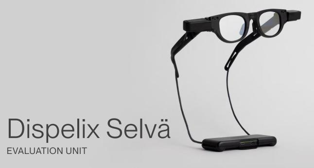
First step to evaluate the Dispelix Selvä LED waveguides
